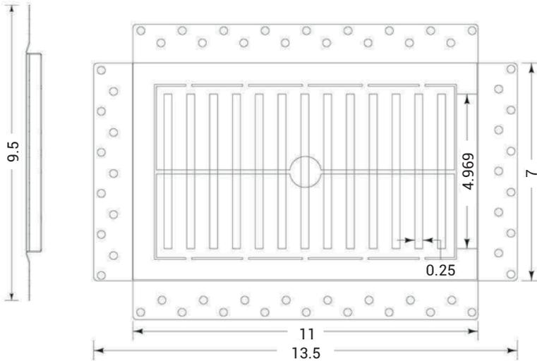
CUT YOUR DRYWALL OPENING TO 11.25" X 7.25" TO FIT THE FRAME INSIDE. CENTER OVER 6x10 BOOT.
