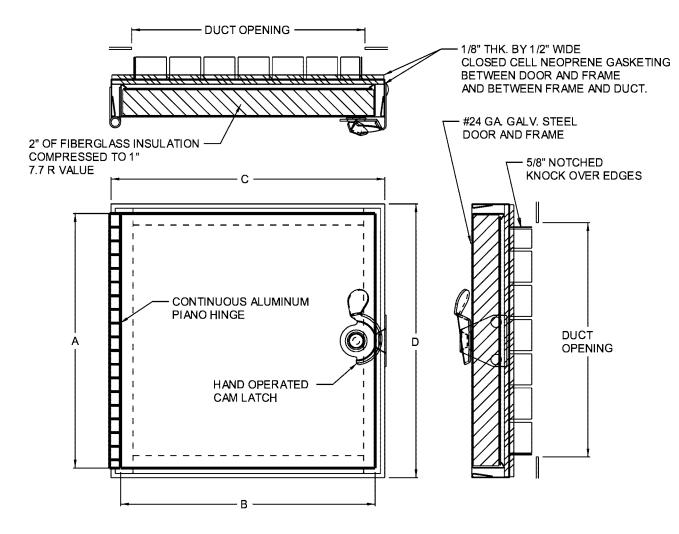
STANDARD FEATURES: HINGED DOOR, SELF TIGHTENING HAND OPERATED CAM LATCH, GALVANIZED STEEL, MILL FINISH.
