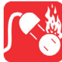
CLASS C FIRES Energized Electrical Equipment
