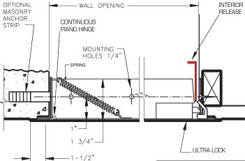
This Premium precision-flush access door for wall and ceiling installation far surpasses other doors. The WB GP 102 Series Premium features close assist, ultra lock and interior latch release.
