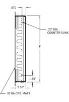
FOR WALLS THIS DOOR HAS A "UL" AND "ULC", 1 1/2 HOUR "B" LABEL, WTH A MAXIMUM TEMPERATURE OF 250 DEGREES AFTER 30 MINUTES. FOR FIRE RATED CEILINGS, THIS DOOR HAS BEEN APPROVED BY WARNOCK HERSEY INTERNATIONAL FOR 3 HOURS (MAX. SIZE 24" x 36").
