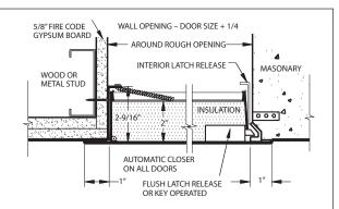
**NOTE:** For fire-rated ceiling access doors, on size  $16" \times 16"$  and larger, extra spring supplied with door must be attached from back of door pan to framing or floor above. In horizontal (ceiling) applications door has self-assisted closing.
