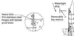
316 Stainless For detailed specifications see submittal sheet steel slamlock D Stainless steel springs 316 Stainless stee Extruded angle automatic hold frame with integral seat & continuous anchor flange open arm with red vinyl grip (25mm)
