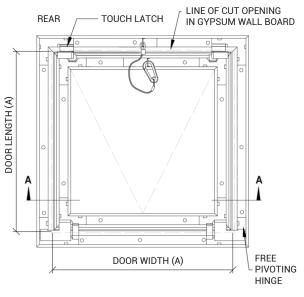
Wall or ceiling opening is W + 2.5" wider and longer than door size, to a maximum of 8"
