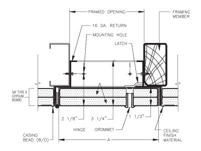
To provide access in a suspended drywall ceiling application that forms part of a fire resistive floor-ceiling assembly. The offset design of the return frame along with a recessed panel with 2 layers of 5/8" Type X Fire-Rated Gypsum board keeps the continuity of the fire resistive quality.
