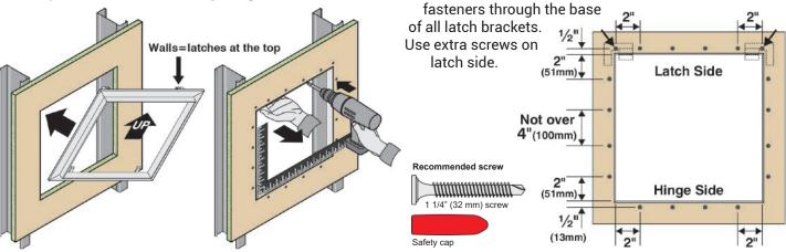
Insert door leaf and test function. Remove. Apply filler into any gaps around the outer frame, filling to the level of the raised edge. Apply filler to the door leaf. Sand and fill until desired finish is achieved. Finished height must not be higher than edge of outer frame and door leaf frame. Setting-type compound is recommended for the first coat. Clean excess filler and dust from frame with a damp cloth.
