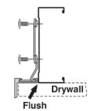
**DURING DRYWALL INSTALLATION** The access panel outer frame can be located resting on the back of
