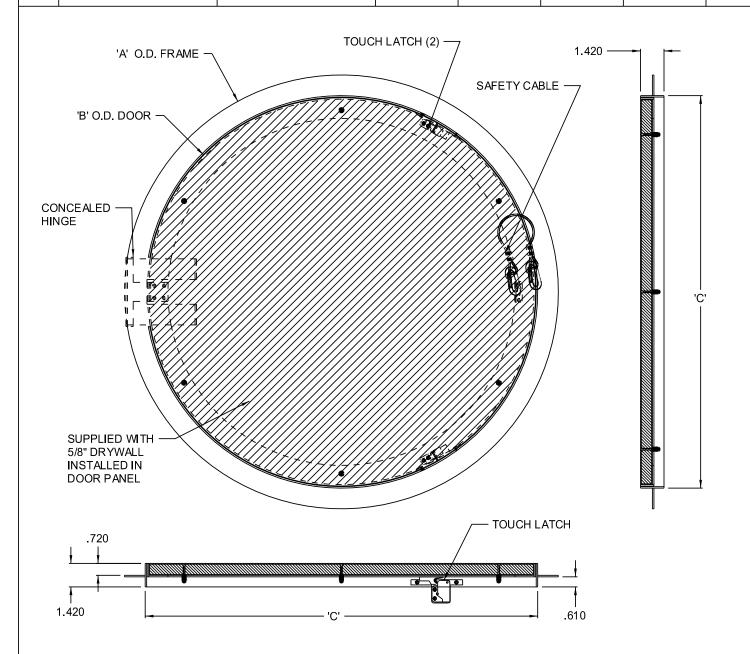
STANDARD FEATURES: TOUCH LATCH; REMOVABLE DOOR PANEL; UNIT IS SUPPLIED TO ACCOMMODATE 5/8" DRYWALL; DOOR PANEL CAN ORDERED TO ACCOMMODATE 1/2" DRYWALL.
