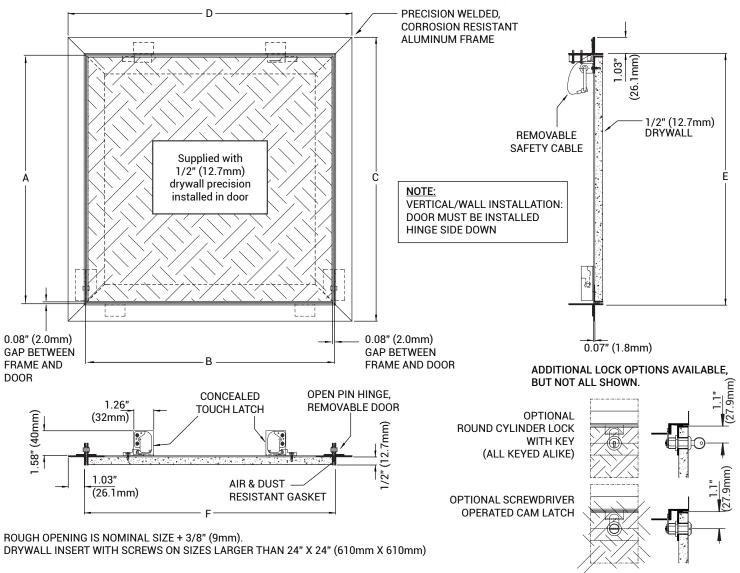
STANDARD FEATURES: CONCEALED TOUCH LATCH; OPEN HINGE, REMOVABLE DOOR; FITS 5/8" (15.9MM) DRYWALL; FOR NON-RATED WALLS & CEILINGS; ALUMINUM FRAME & DOOR STRUCTURE, WELDED, MILL FINISH; NON-SNAG REMOVABLE SAFETY CABLE
