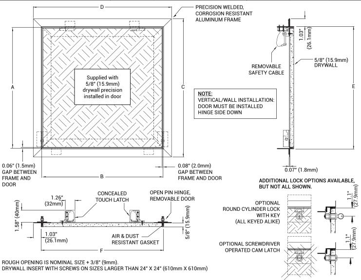
STANDARD FEATURES: CONCEALED TOUCH LATCH; OPEN HINGE, REMOVABLE DOOR; SUPPLIED TO FIT 5/8" (15.9MM) DRYWALL; OR NON-RATED WALLS & CEILINGS; ALUMINUM FRAME AND DOOR STRUCTURE, WELDED, MILL FINISH; NON-SNAG REMOVABLE SAFETY CABLE
