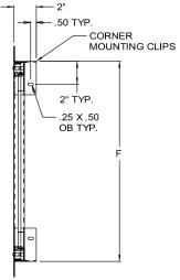
The WB ADWT is a flush access door that has been tested for air infiltration and water penetration. The Door and frame are fully welded and gasketed. This access door is ideal for use in laboratories, clean rooms, operating rooms, etc. where an airtight/watertight seal is required.
